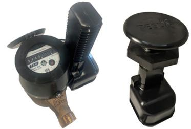
**Activation:** Tesla Solo endpoints are shipped in an inactive, non-transmitting state. After installation, the endpoints begin communicating data once the encoder indicates water has been used. Alternatively, a magnet can be used to manually activate the endpoints and verify the encoder connection.
